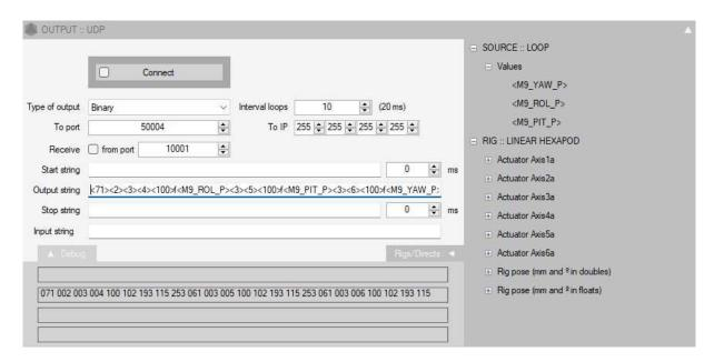
After pressing 'Connect', the platform will roll, pitch and yaw according to the sine pattern.
