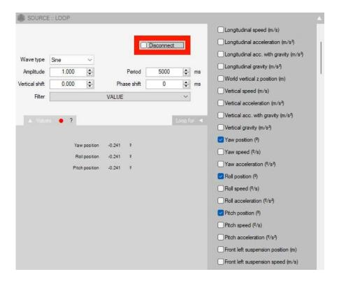
Then, the parameters <M9\_YAW\_P>, <M9\_ROL\_P> and <M9\_PIT\_P> can be assigned to axes 4, 5 and 6 respectively as platform position (<mode\_AxisXX> = 3), as follows:
